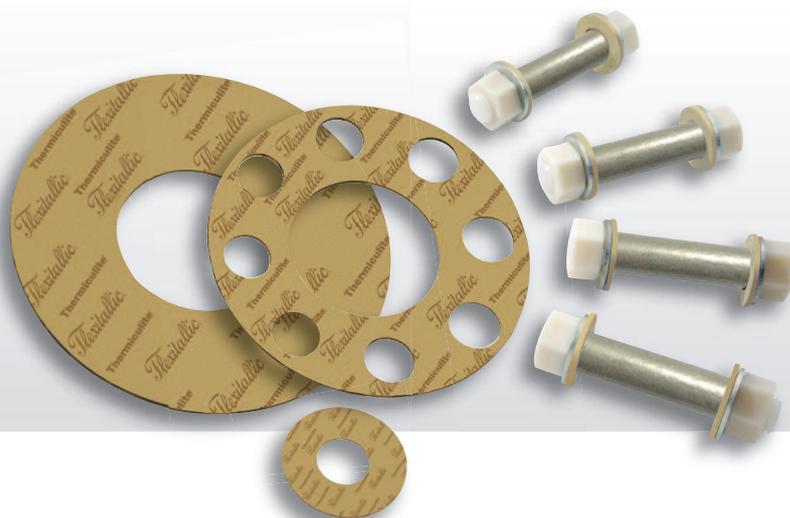
The Flexitallic I-Flex Fire-Safe Flange Insulating Set (FS-HP) is comprised of a fire safe insulating gasket, insulating sleeves, insulating washers and metal backing washers.
